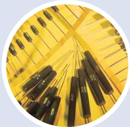
Our wirewound resistors feature an alloy resistance wire precision-wound to a heat-conducting ceramic substrate, with welded endcaps and lead terminations, and silicone conformal coating protecting the resistive element.
