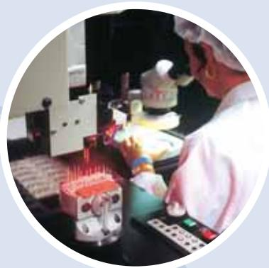
IRC's class 100 clean room allows the latest in thin film technology to produce a series of TaNfilm® surface mount resistors and TaNSil® resistor networks that are widely used in military/aerospace, commercial and precision applications.
